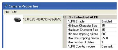
The field ALPR Enable must be set to "Enabled".
